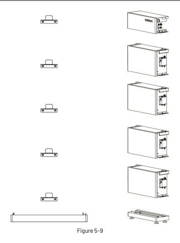
11. Secure the RBSs each other and BMC with RBS using M5 screws.
